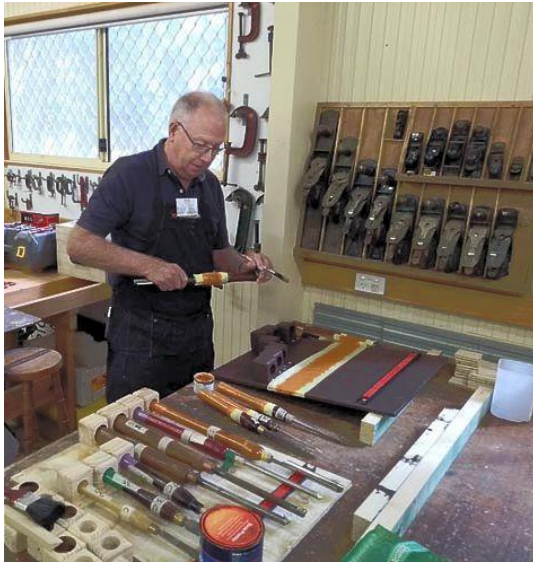
Dick is making a magnetic lathe tool rack to hold gouges and tools for each wood lathes
