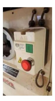
Please take care when using our machinery. John Beales has again repaired the red off / reset button of our main saw table with the pink slide. This button no longer needs to be twisted prior to pressing the green "on" button.
