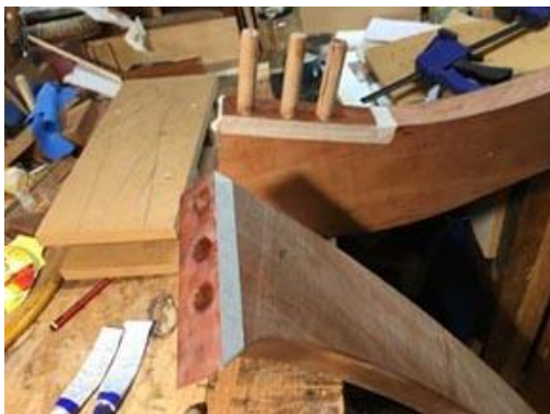
Neck and pillar templates. Plank: Tasmanian leatherwood 235 x 43 x 1900
