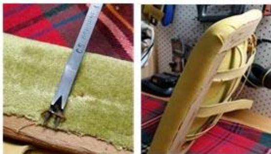
This meant taking out a large number of old staples. This isn't a job for a screwdriver or small chisel as you will invariably make a mess of the fabric and timber seat frame.
