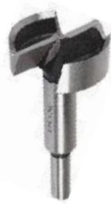
Forstner bits have radial cutting edges to plane off the material at the bottom of the hole. The bits shown in the image has two radial edges; other designs may have more.
