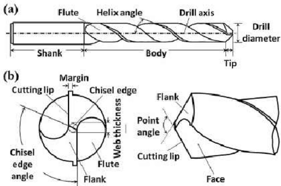
A more aggressive angle, such as 90 degrees, is suited for very soft plastics and other materials but it would wear rapidly in hard materials. Such a bit is generally self-starting and can cut very quickly. A shallower angle, such as 150 degrees, is suited for drilling steels and other hard materials.
