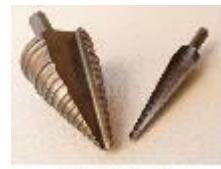
Step drills are commonly used on sheet metal and in general construction. They are often used on softer materials, such as plywood, particle board, drywall, acrylic, and laminate. They can be used on very thin sheet metal, but metals tend to cause premature bit wear and dulling.
